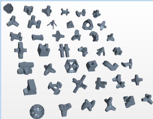
The protection blocks, are some structures that are placed in zones near Ports mainly, with the objective to mitigate or to eliminate the energy that contains the continuous wave: there are a lot types or models: x-blocks, Accropodes, Tetrapods, Cubipods, etc....
