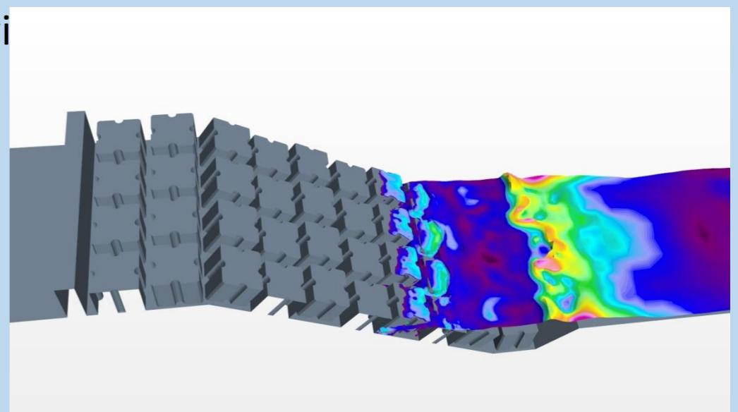
From pressure distribution in every element, we are able to calculate the structure forces (from water pressure and elements weight forces), in order to know the fatigue and stress. This analysis is based in Finite Elements:
